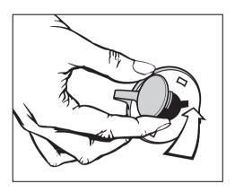
■ Fit the covers on to the two holes. Then plug the holes as shown with the caps. The washing machine must not be moved without the transit bars in place.
